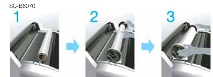
Place the paper roll above the groove on the top of the printer
